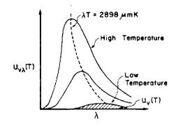
Fig. IIID-1. The Energy Distribution of Thermal Radiation
